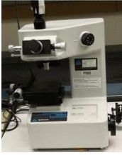
Buhler Micromet automatic computer controlled microhardness tester
