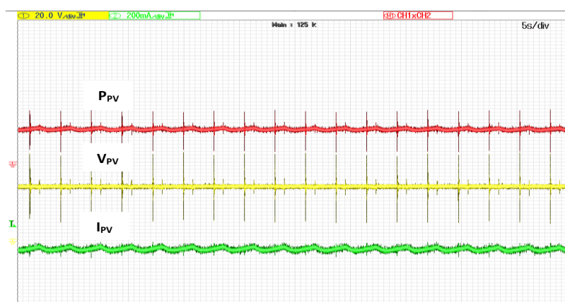
Figure 5-8 PV array power, voltage, and current waveforms at the MPP with 4 W/div, 20 V/div, and 200 mA/div respectively, and with a perturbation size of 0.01.
