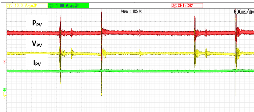
Figure 5-6 PV array power, voltage, and current waveforms at the MPP with 10 W/div, 10 V/div, and 1 A/div respectively, and with a perturb size of 10^{-7} .
