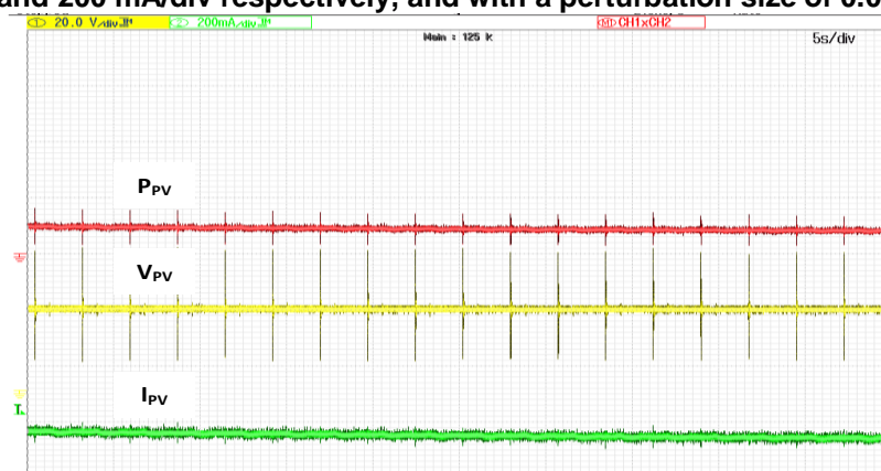
Figure 5-9 PV array power, voltage, and current waveforms at the MPP with 4 W/div, 20 V/div, and 200 mA/div respectively, and with a perturbation size of 10^{-7} .
